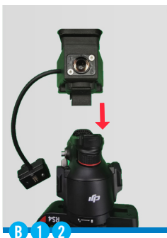
Attach Head unit module to Ronin
