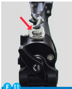
Front steel tension cable hang
