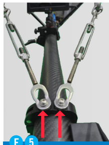
Rear steel tension cable hang
